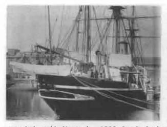
HMS Condor was a barque-rigged twin screw steel steam sloop. Although some sources give her rig as barquentine or brigantine a photo of the ship, first of her class, shows that she was barque rigged. Sisterships were later rigged as barquentines or brigantines to reduce sail area after the loss of Condor; all had their sailing rig removed within a few years. She was a new ship, having been launched at Sheerness in December 1898 and
